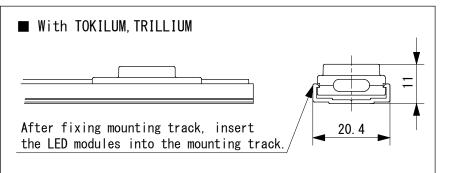
The length of Mounting Track is fixed 1.25m. It can be cut on job site.
