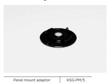
The socket assembly is inserted from below and the panel mount adaptor is pressed in place from above. Provide a Φ54mm hole to install the socket. Recommended spacing between the holes is 250mm in consideration of wiring.
