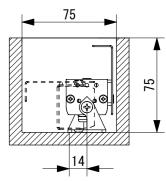
When tilting an extrusion 90°, the minimum installation space is shown above and offset the center axis of the fixture installation by about 14mm.
