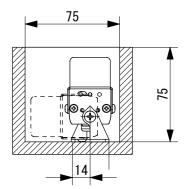
When tilting an extrusion 90° the minimum installation space is shown above and offset the center axis of the fixture installation by about 14mm.
